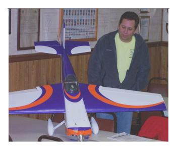
It is built from a D&L Designs kit. It took about 3 months to build at a leisurely pace. Tech spec's: 60" span / 7 pounds. It's a standard 4 channel / 5 servo setup, but he chose to use a second aileron channel instead of a Y harness. Just cause he can (something new to try on his Futaba 9CAP Super). He did a 'build along' on RC universe. Can't wait to see this baby move come spring!
