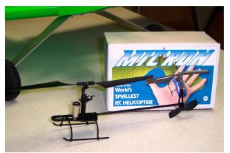
Jim Fassino's Precision Heli Micron helicopter. It weighs less than 2 ounces A.U.W. and flies with a four channel radio and gyro. It is the smallest production heli. "It's Maiden flight was great. Small heli but big smile." (I'll have to see it fly to believe it.)
