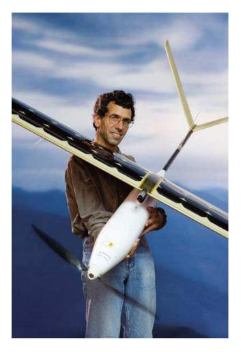
Powered by solar cells, Alan Cocconi's SoLong remained aloft for two days. Some engineers are hopeful that aircraft like SoLong could be used as "radio towers in the sky."
