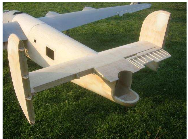
Tail view showing features for internal hinges. Wes buries the pivot rod end, after painting, with putty and touch up paint.
