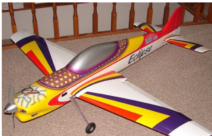
Shown above is Bob Wilson's new Eclipse pattern aircraft. The airframe is made from composite materials and has a YS motor.
