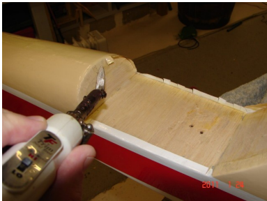
Using the hot trim iron to "roll over" the tabs.
