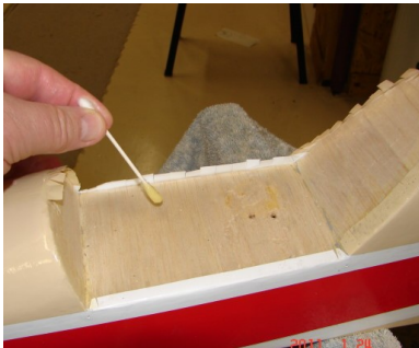
Applying contact cement to the cockpit area. Note the Monokote tabs.
