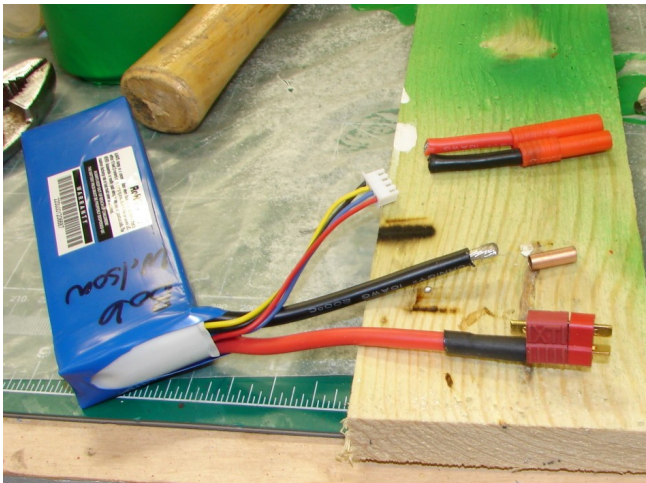
Cut one lead and trim back the insulation 1/4". Cut a 5/8" piece of 3/16" OD copper tubing.
