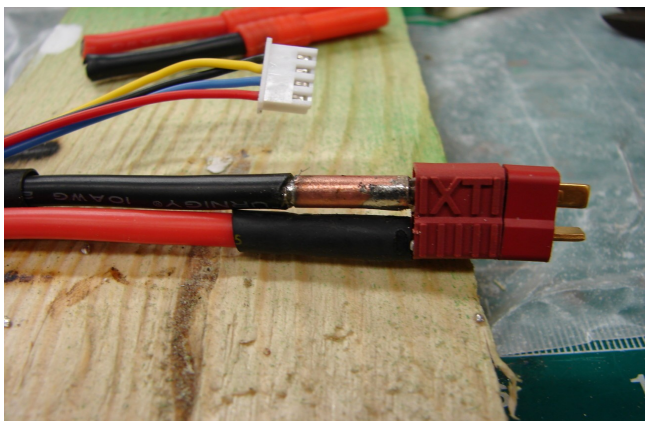
The 3/16" OD copper tube will just slide over the Deans tab. Leave about 1/16" between the copper tube and the base of the plug. Heat and run solder into that opening.
