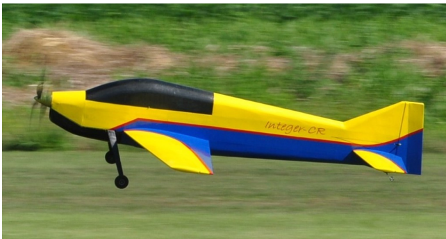
Mike Gaishin's unique "contra" on landing. This is an electric powered airplane w/ counter rotating props.
