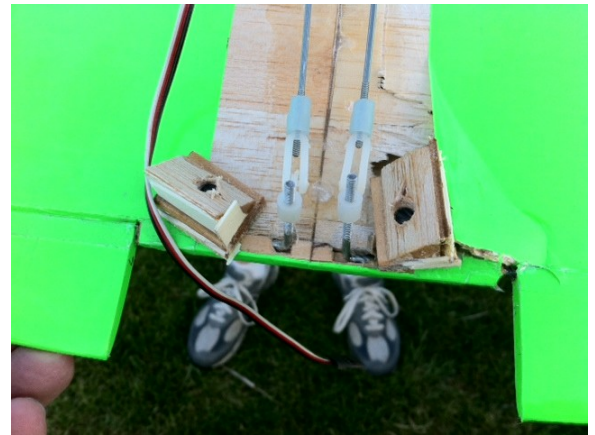
Part of the result of a severe stall on take-off initiated by engine failure. I've never seen little feet on a wing before! (Editor)
