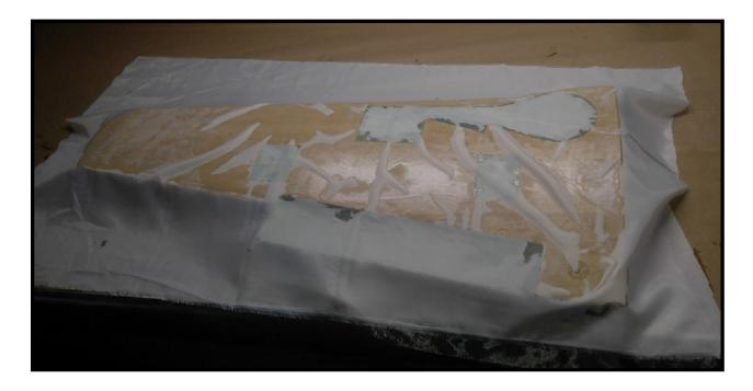
Drape the peel ply across the wing over the cloth and start working in down with the card, working from the middle out. I skipped ironing this piece for some reason.
