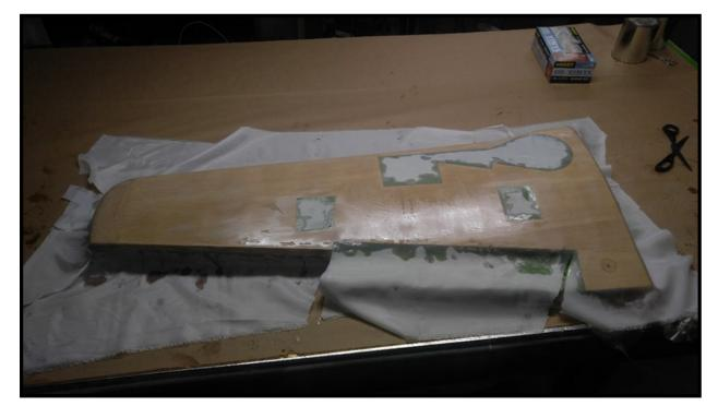
If you have any dry looking spots, brush on a little resin and continue to squeegee out as much resin as you can. The peel ply should be saturated across the entire surface.
