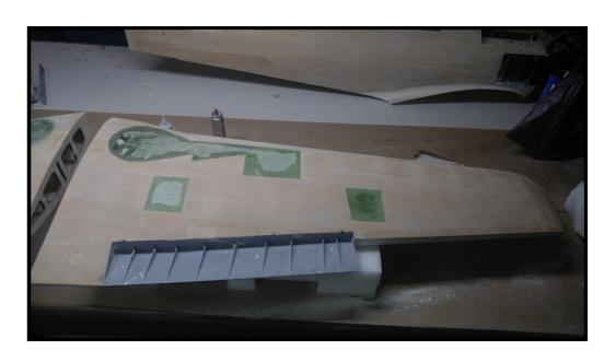
Here is the magic of the whole process. Once cured, the peel ply peels off and leaves a very smooth surface that can quickly be sanded out with some 220 grit paper. No second coat, no sanding in between, and no toilet paper mess all over the place and creates a nice uniform surface to prime and paint on.
