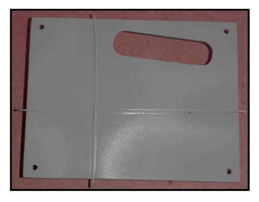
Shoot 3 or 4 coats of Filler Primer over the tape lines and let it cure up for a couple of days. I didn't have a couple of days here so I flash dried it with a heat gun. After it's dry, lightly sand to expose the top of the tape and remove it.
