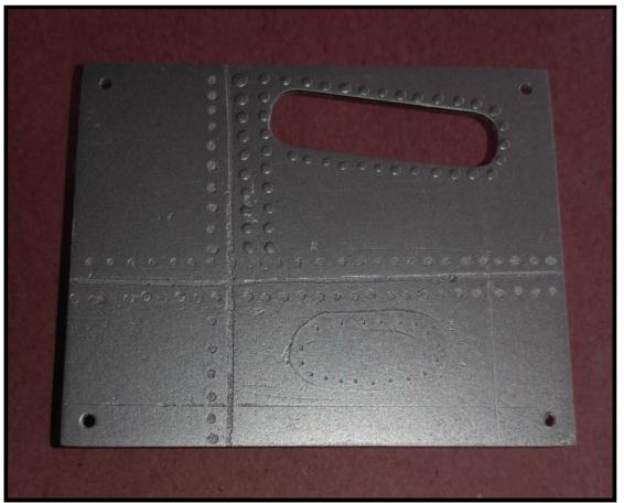
Here, the panel is sprayed with a silver base and all the little details are really popping out. At this point, the piece is ready to be weathered and cleared. This is an active test panel in the shop right now and from this point I am trying a couple more new techniques. Stay tuned!
