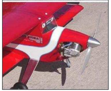
(Left) Hal DeBolt's "Live Wire". Built by Lyman Slack. A 70 powered 4 cycle pulls this 7.5 lb, 66 inch span, vintage biplane. Love that see-thru red! Don't you?! And the striping the feathers in to the landing gear for the finishing touch.
