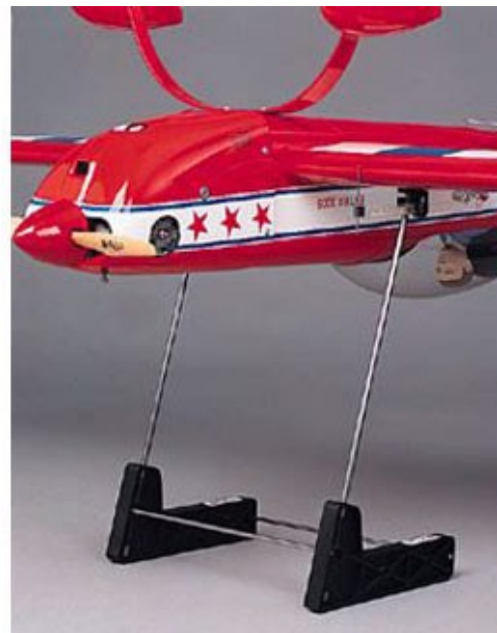
(Above) The GP Balancer is a great tool to have in your workshop. Du-Bro Stick on weights are excellent for adding nose weight.
